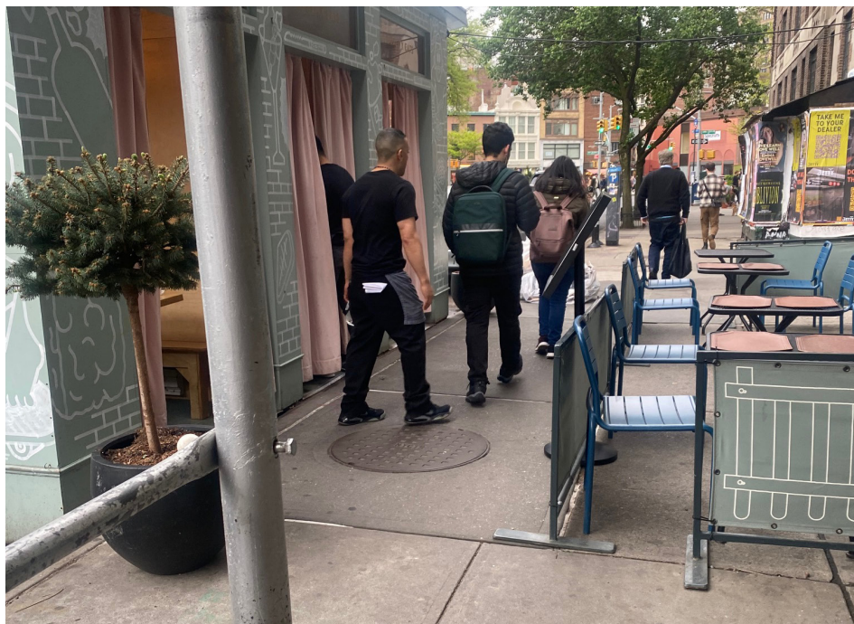
Note obstacle course, and well under 8-ft clear path exacerbated by planters.
